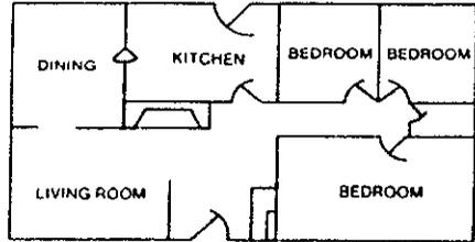
In homes with more than one sleeping area a smoke detector should be provided to protect each area. Smoke detectors shall be located between the sleeping area and the rest of the house. **NOTE:** Refer to N.F.P.A. 874 Appendix B1.1 through B-10.
